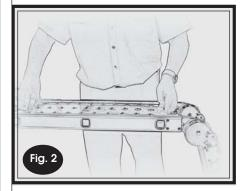
Lower the deck until it lies flat, (Fig. 2) with the lip pushed up to the first ladder rung. The other end of the deck should be covering half of the rung it is lying on.
