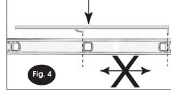
Fig. 4 shows correct alignment of lip and lugs to prevent sideways movement.
